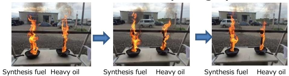
The synthesis fuel is completely burnt and less black smoke.
